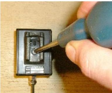
First, remove the existing mounting bracket from the light, if it has one. This photo shows a Solidlights handlebar bracket fitted to a 1203D. Also remove any gaskets under the bracket.
