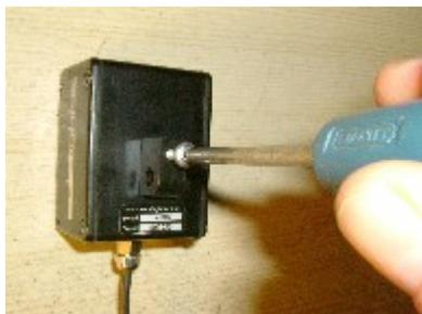
Next, use the supplied M4x25mm screw to attach the adapter block to the light. Note the orientation: in most cases, it is best to put the curved part of the adapter block towards the rear of the light, as this provides most clearance for the cable.
