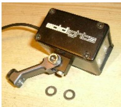
Now assemble the adapter and light to your bracket using the M6 screw and nut. Since the walls of brackets vary in thickness, two washers are provided to fill any space if required. In the case shown they are not necessary.
